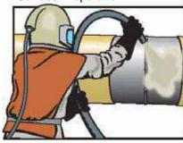
4. Blast clean surface to a near white ISO-8501, NACE No. 2, SA-2 1/2 (SSPC-SP 10) or better using particle blasting (sand or other). Sweep blast adjacent FBE coating 50 mm (2") to either side of bare steel area (cutback).
