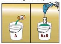
7. If necessary, warm parts A and B to 20° C (68° F). Agitate part B before mixing. Mix by pouring all of part B into part A. Thoroughly scrape container and lid of part B. Slowly begin mixing to avoid introducing air into the mixture.
