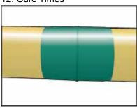
12. The curing rate will vary according to pipe and ambient application temperature. Refer to Cure Chart to determine when to perform a shore D check.
