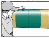
11. Use a wet mill gauge to measure that the desired minimum thickness has been achieved. Double check around the weld to insure minimum desired thickness.
