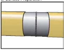
5. Establish a 2.5-4 mils (64-100 microns) surface profile with sharp angularity. Burnishing or polishing must be avoided. Surface preparation can be controlled using surface profile tape. Dry surface and insure ideal surface preparation.
