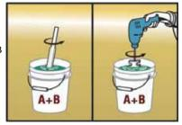
8. Use mixing speed that uniformly blends the 2 parts, but doesn't create a vortex in the mixture or spillage. Blend both parts to create a uniform color with no streaks.
