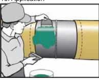
10. Use trowel, brush or roller to apply required minimum thickness of coating. Cover at least 50 mm (2") of the adjacent mainline coating.
