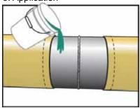
9. Reconfirm that the application temperature is above 10° C (50° F) and 3° C (5° F) above dew point. Slowly pour mixed epoxy onto the pipe. Apply thin film evenly to wet out substrate, then build coating to desired thickness. If the pipe is heated before and during application, R65-F-1 can be applied at temperatures below 10° C (50° F).
