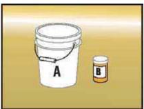
1. The two component epoxy coating is supplied in premeasured kits. Part A (large container) is the base and Part B (small container) is the curing agent.
